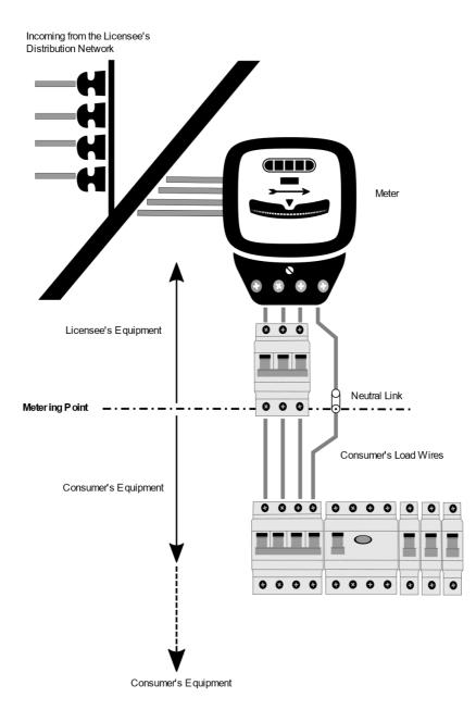
*Note*: Shown here is the typical set-up for a three-phase installation. A Single-phase installation will have appropriate lesser number of poles in respective MCBs.
