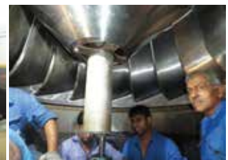
New nose cone fixed to the runner
