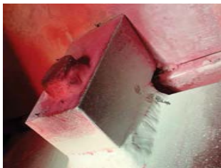
Pole stopper with crack
