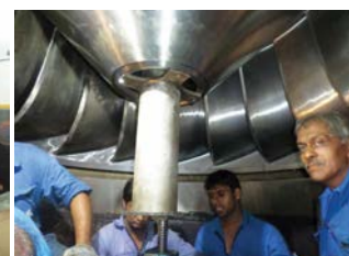
New nose cone fixed to the runner
