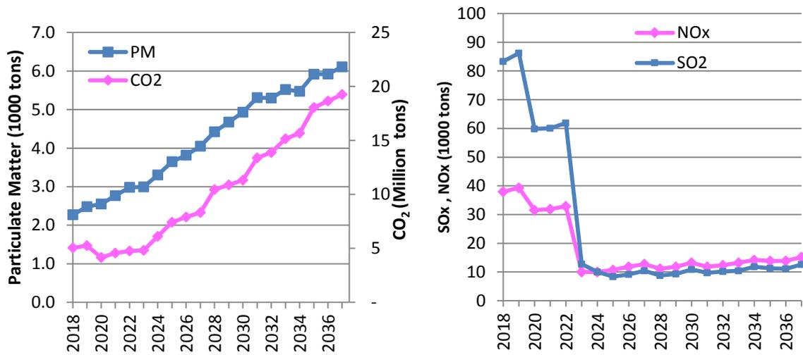
Figure 9.4 – PM, SO<sub>2</sub>, NO<sub>x</sub> and CO<sub>2</sub> emissions of Base Scenario
