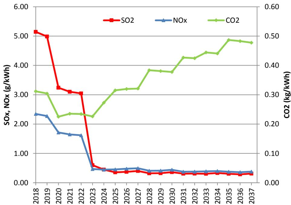
Figure 9.5 – SO<sub>2</sub>, NO<sub>x</sub> and CO<sub>2</sub> emissions per kWh generated
