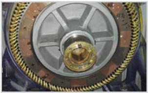
Replacement of bearings of traction motor- No 02 Boiler lift-LVCPP
